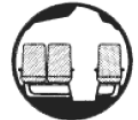
SF-340 Aisle Height 6' 0" Max Width 7' 1"
