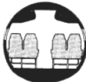
DHC-8 Aisle Height 6' 0" Max Width 8' 2"
